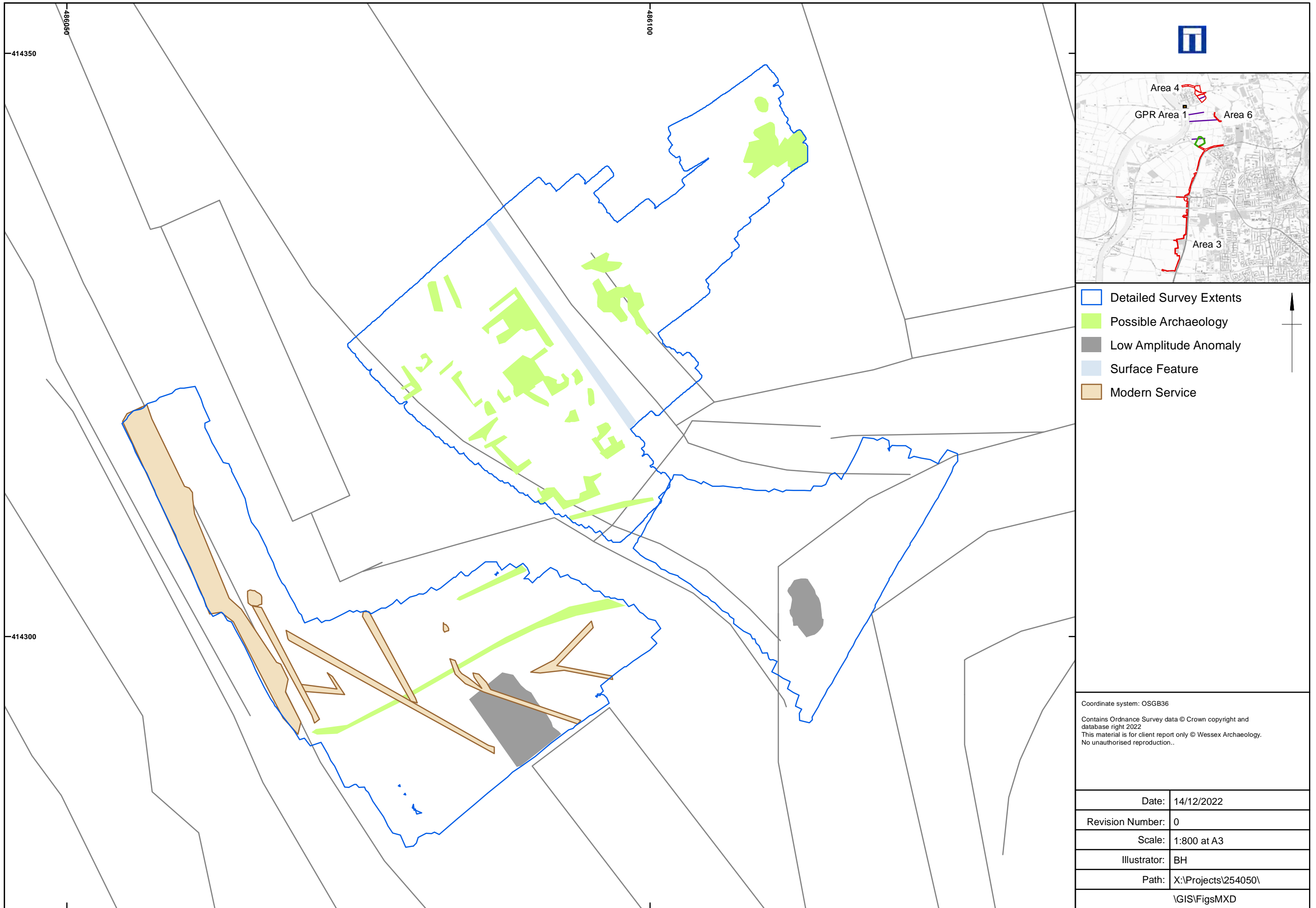
Ground penetrating radar survey results:overall interpretation
